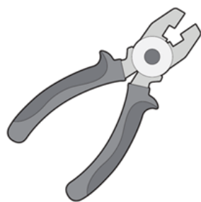
Wire-stripping tools for stripping 6-AWG copper wire
