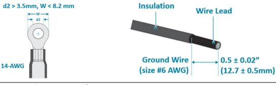
14-AWG wire with ring terminal for DC power supply
