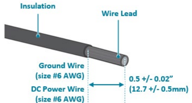
6-AWG green-and-yellow wire for grounding 6-AWG DC power wire
