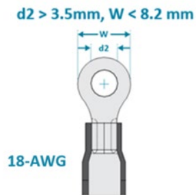
18-AWG wire with ring terminal for DC power supply
