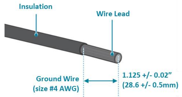
4-AWG green-and-yellow wire for grounding
