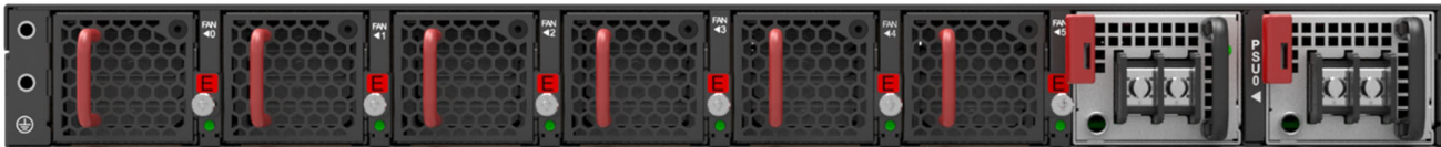
(Front-to-Back Airflow Fans)
