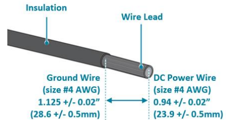
4-AWG green-and-yellow wire for grounding 4-AWG for DC power wire
