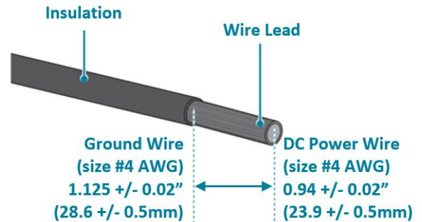
4-AWG green-and-yellow wire for grounding 4-AWG DC power cable
