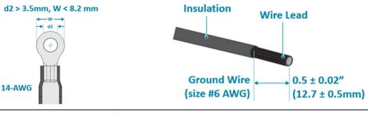
14-AWG wire with ring terminal for DC power supply
